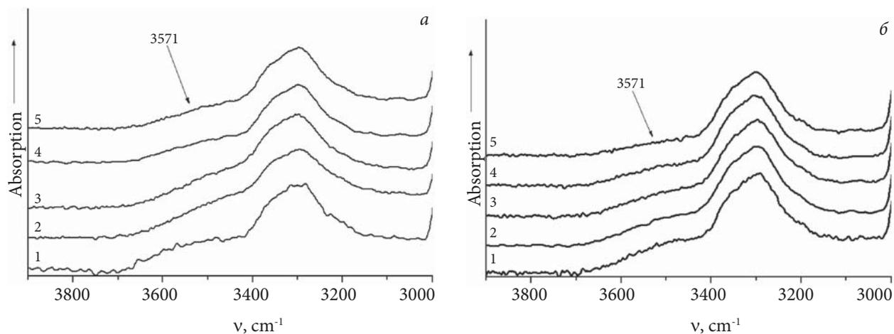
**Fig. 2.** Fragments of IR spectra of PUF composites with albugid before and after incubation in BM 199 (a) and saline solution (b) for 2 weeks (2), 1 month (3), 3 months (4), 6 months (5) in the range of 3000–3800  $\text{cm}^{-1}$
