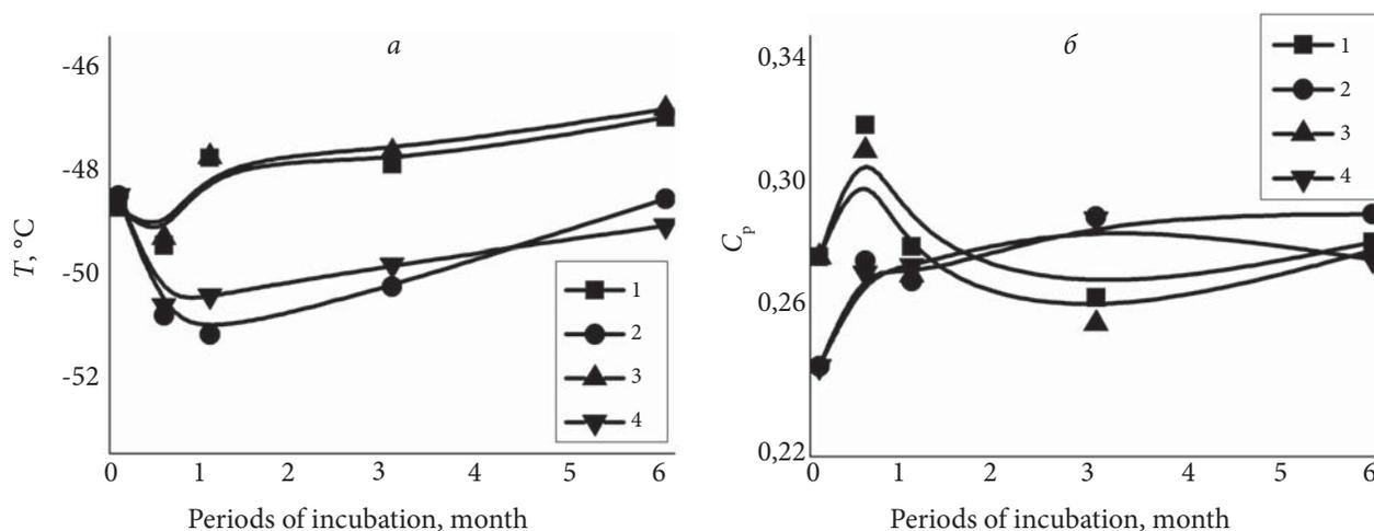
**Fig. 3.** Dependence of glass-transition temperature (a) and heat capacity (b) of PUF (1, 3) and PUF composites with albucid (2, 4) on the term of their incubation in BM 199 (1, 2) and saline solution (3, 4) (2nd heating procedure)
