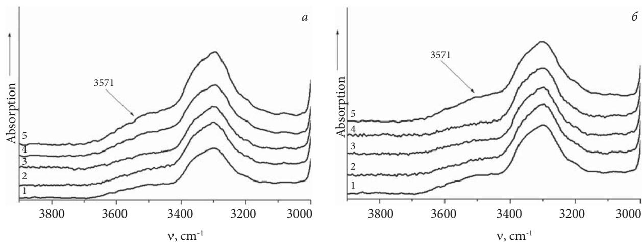
**Fig. 1.** Fragments of IR spectra of PUF before (1) and after incubation in BM 199 (a) and saline solution (b) for 2 weeks (2), 1 month (3), 3 months (4), 6 months (5) in the range of 3000–3800  $\text{cm}^{-1}$
